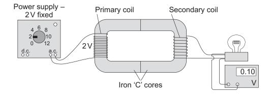
**1 (a)** The transformer made by the student would not have worked if the core had been made from aluminium and not iron.
