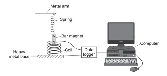
**3 (a)** Explain why the ground vibrations cause an electric current to be induced in the coil. The first sentence of the explanation has been done for you.
