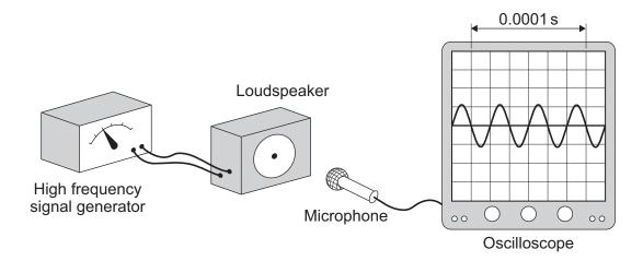
5 (a) (i) How many waves are produced by the loudspeaker in 0.0001 seconds?
